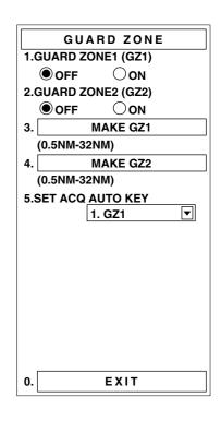
Note: Guard Zones 1 or 2 can be set in any area within a range of 0.5 to 32 NM.
