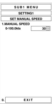
Note: The manually entered speed is effective only when 1. MANUAL is set in 2.SELECT SPEED.
