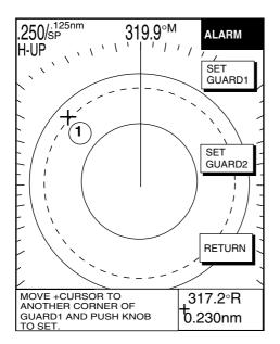
Drag cursor to top (or bottom) corner for guard zone and press the SET GUARD1 or SET GUARD2 soft key.
