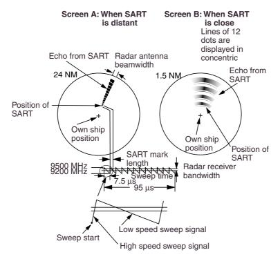
Appearance of SART signal on the radar display
