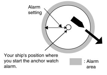
How the anchor watch alarm works
