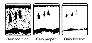
Examples of proper and improper gain
