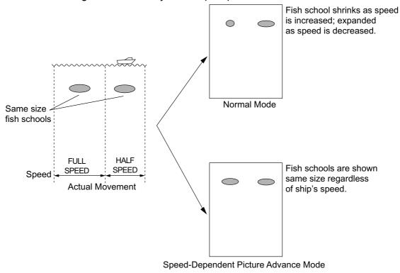
How the speed-dependent picture advance mode works
