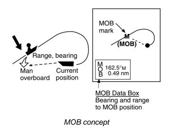
Press and hold down the SAVE/MOB key for about three seconds when someone falls overboard. The display shows the waypoint number being saved (youngest empty waypoint number, 001-999) followed by the MOB confirmation window. Time remaining is counted down while pressing the SAVE/MOB key.
