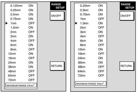
\* = Max. range depends on network radar used and is set on the network radar at installation. <u>Range unit: nm</u> <u>Range unit: km</u>
