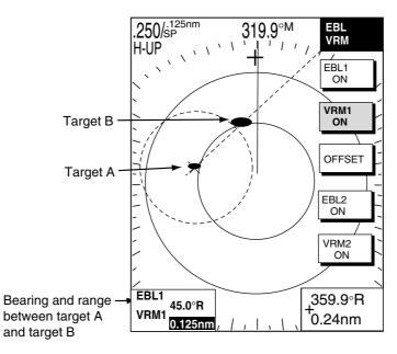
Measuring range and bearing between two targets
